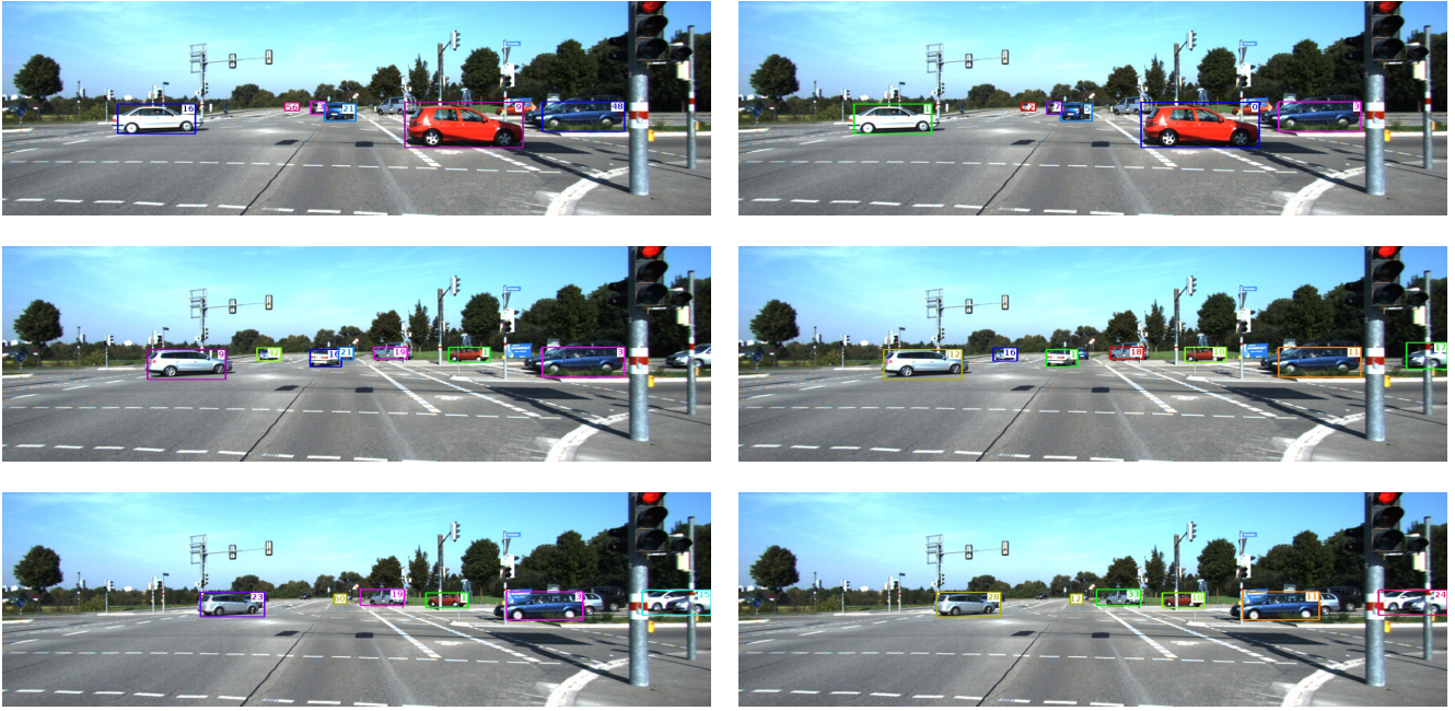
Figure 12: Qualitative Results for the Optimal (left) and our Approximate Solution (right). Challenging intersection scenarios lead to qualitatively good results. The limited optimization window for the approximate solution may also prevent changes for parts of trajectory outside of this window. Due to this approximation, track 9/12 is not fragmented for mbodSSP.
