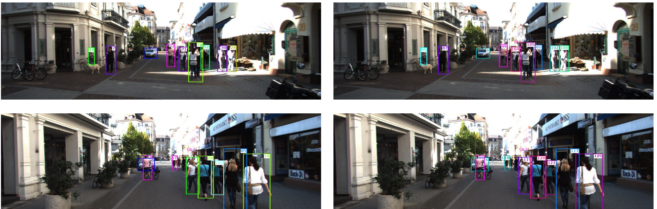
Figure 15: Qualitative Results for the Optimal (left) and our Approximate Solution (right). For groups of interacting pedestrians, tracks are correct even for partly occluded objects. Very high occlusions for several frames may lead to interrupted tracks.
