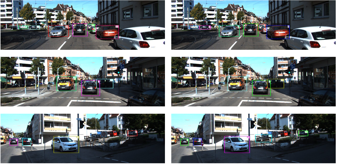
Figure 10: Qualitative Results for the Optimal (left) and our Approximate Solution (right). Preceding objects in crowded scenes are well tracked. Track 3/1 is followed for 9.5s
