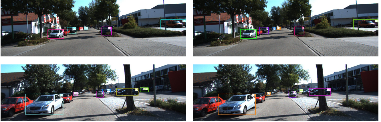
Figure 8: Qualitative Results for the Optimal (left) and our Approximate Solution (right). Far away objects are well tracked. Track 13/11 is followed for 3.7s and not confused with several parking cars.
