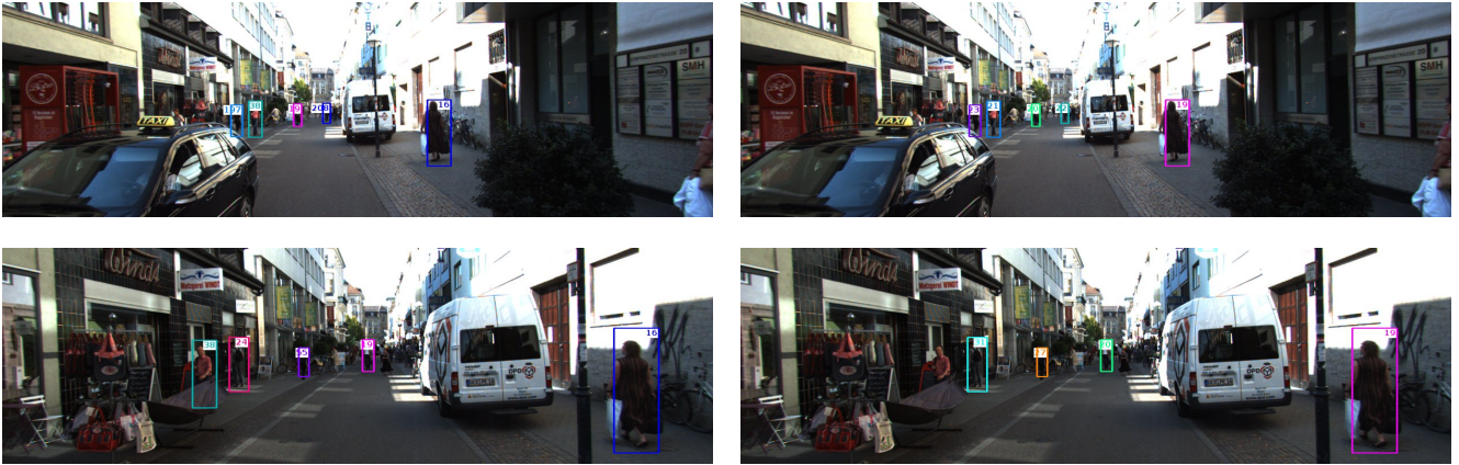
Figure 14: Qualitative Results for the Optimal (left) and our Approximate Solution (right). For crowded inner-city scenes, objects of different classes (cars, pedestrians, cyclists) are tracked robustly.
