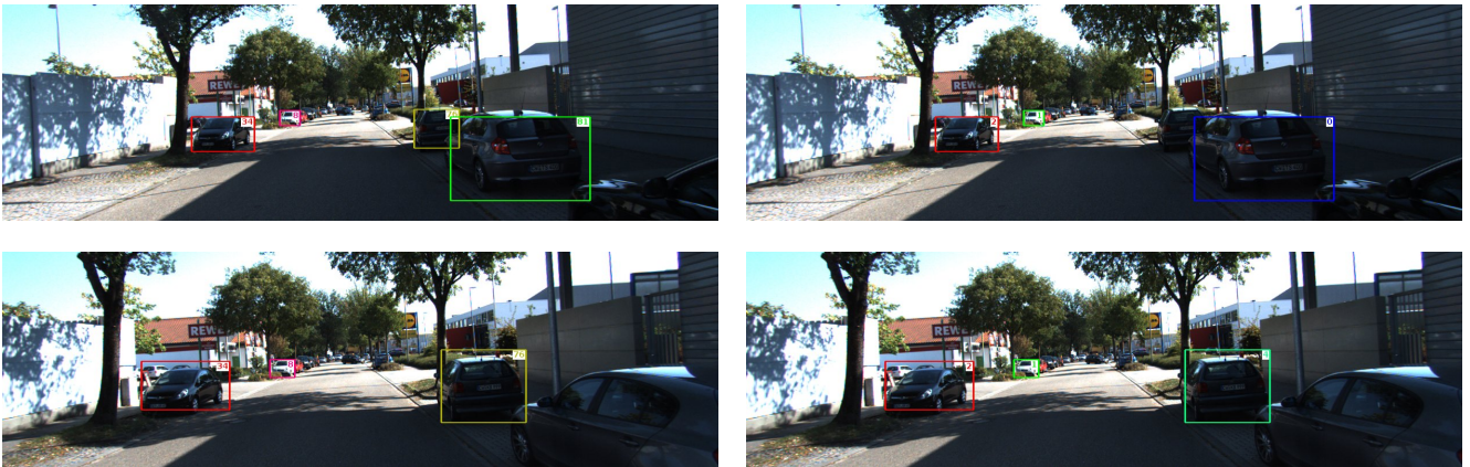
Figure 13: Qualitative Results for the Optimal (left) and our Approximate Solution (right). Missing future evidence for the approximate solution may lead to tracks that start later when compared to the optimal solution (track 76/4). This happens primarily for detections with a low score for the early part of the trajectory.
